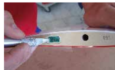
64. ...v pásce vyřízneme otvor pro protikus konektoru... ... cut hole in the tape for complemented connector ...
