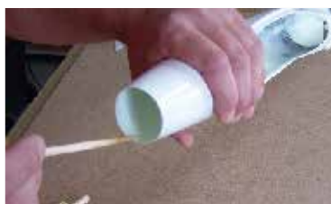
108. ...nanese me lepidlo... ... put glue on the surface ...
