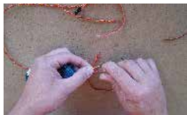
115. ...kabely odizolujeme a pocínujeme... ... cut insulate and solder end of the cable ...
