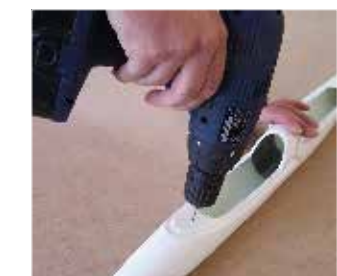
75. ...vyvrtáme otvor Ø2,2mm... ... drill hole ø 2.2 mm ...
