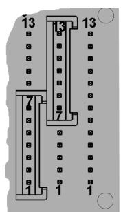
available for order. Thus any combination to connect an accupack can be realized. The third row of holes can be used to connect other plug systems by soldering the adapter cables to it. Although the UNI board can be used for different connecting systems, we recommend to use specifically configurated UNI boards for each application. Only this guarantees a maximum of safety.
