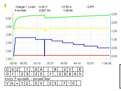
Charging ends when threshold voltage is detected and simultaneously charging current is decreased. When *Fast* mode is on charging current is controlled with pulses, which makes it possible to reduce charging time more than two times. Current limitation can occur when voltage overstep maximal value for given cell types. We recommend the *Pulsar EQUAL* Equalizer from ELPROG.
