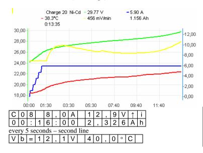
C 08 - charging; 8 cells 8,0A - actual, measured current 12,9V - actual, measured voltage ↑ - marker of increasing voltage
