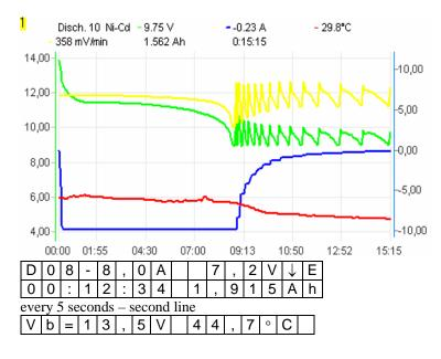
Discharging lasts until battery voltage reaches threshold voltage for given cell type. In *Auto* mode current is decreased by ½ each time the threshold voltage is reached. Discharging process ends when discharging current is less than 200mA. *Reverse* mode – energy from discharging battery is transferred back to the supply
