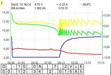
10,00 Discharging lasts until battery voltage reaches threshold voltage for given cell type. In Auto mode current is decreased by ½ each time the threshold voltage is reached. Discharging process ends when discharging current is less than 200mA. Reverse mode – energy from discharging battery is transferred back to the supply car battery.
