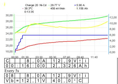
Charging ends when voltage drop (- $\Delta v$ ) or inflex point is detected.
