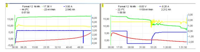
Formatting a battery means to perform demanded number (1 to 8) of discharging-charging cycles. Discharging is performed in *Auto* mode until threshold voltage is reached, which depends of cell type. Reconditioning a battery – special formatting mode which allows repairing the battery.
