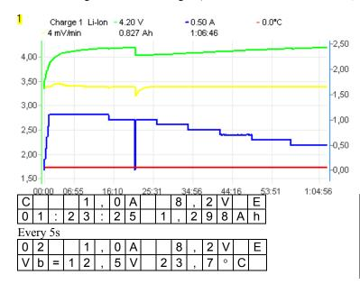
Charging ends when threshold voltage is detected and simultaneously charging current is decreased to 1/10-th (1/5-th for PB-bat) of adjusted value. When *Fast* mode is on charging current is controlled with pulses, which makes it possible to reduce charging time more than twice. Current limitation can occur when voltage overstep maximal value for given cell types.
